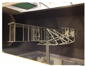
The 4 ft wingspan model mounted in OSU's 5 ft tunnel and almost ready for action.
