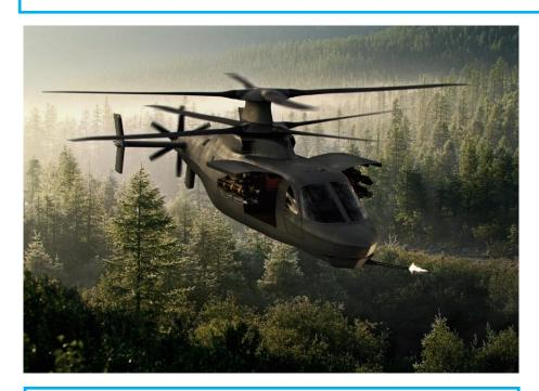
An artist's concept of Sikorsky's Raider X, a candidate for the US Army's Future Attack Reconnaissance Aircraft (FARA). The Army calls it a "knife fighter" on the battlefield of the future. Sikorsky's X2 technology, proven in flight, includes rigid, counter-rotating blades, fly-by-wire flight controls, and an integrated auxiliary propulsion system that will push the aircraft at 250 knots! Raider X is one of 5 designs in competition. The field will down-select to two for a "fly off" in 2023.
